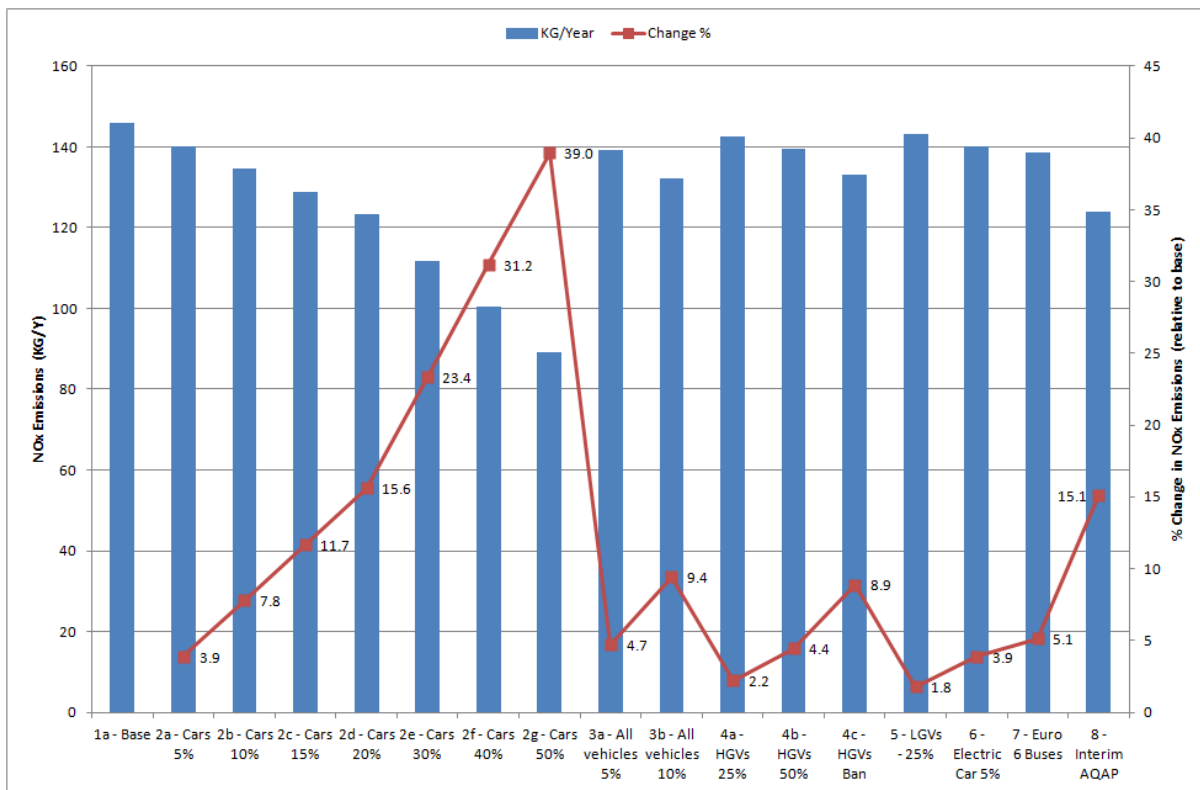
Figure 10: Changes in annual NO x emissions (KG/Y) under each scenario (2018 modelled year)
